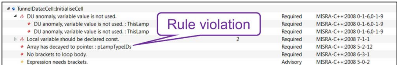
Figure 3: Highlighting violated coding rules and guidelines in the LDRA tool suite
